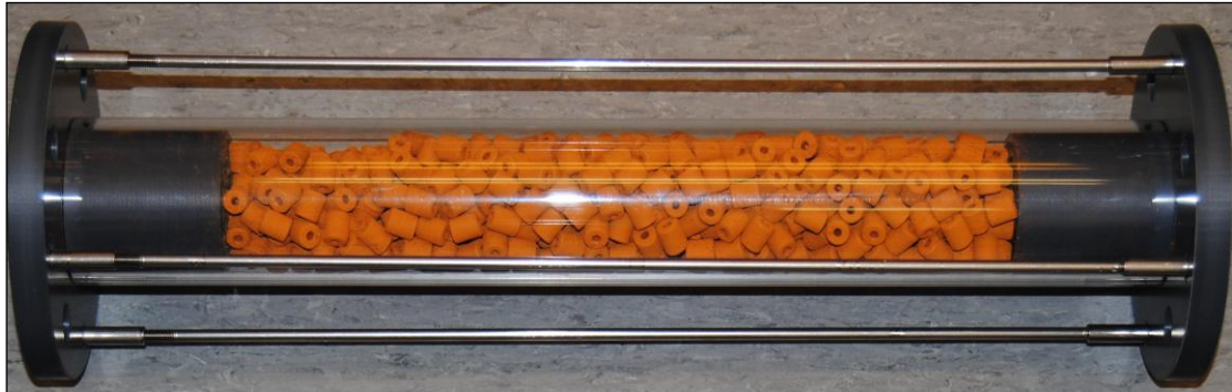
Figure 1. Example of a purification unit used in the trial
